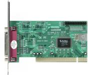
The LCS-6020 is a Multi I/O Controller Card for the PCI-Slot. Today more and more Mainboards come without an Serial- or Parallel-Port, the LCS-6020 is the solution and will give you the needed ports. The Adapter is usably for Printers, Machine-Steering or other Devices.
