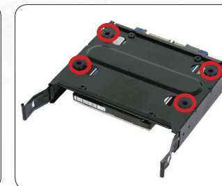
Mounting of 2.5 inch drives (3.5 inch sled)
