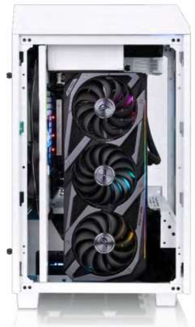
Maximum VGA length: 330mm
