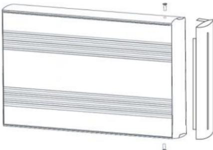
**English :** Remove the screws on the side and remove the back panel.
